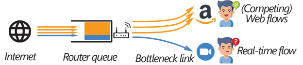
Fig. 2: The scenario where the real-time flow is affected by competing flows. When Web flows join the competition with the real-time flow, the available bandwidth of the real-time flow will be immediately reduced.
