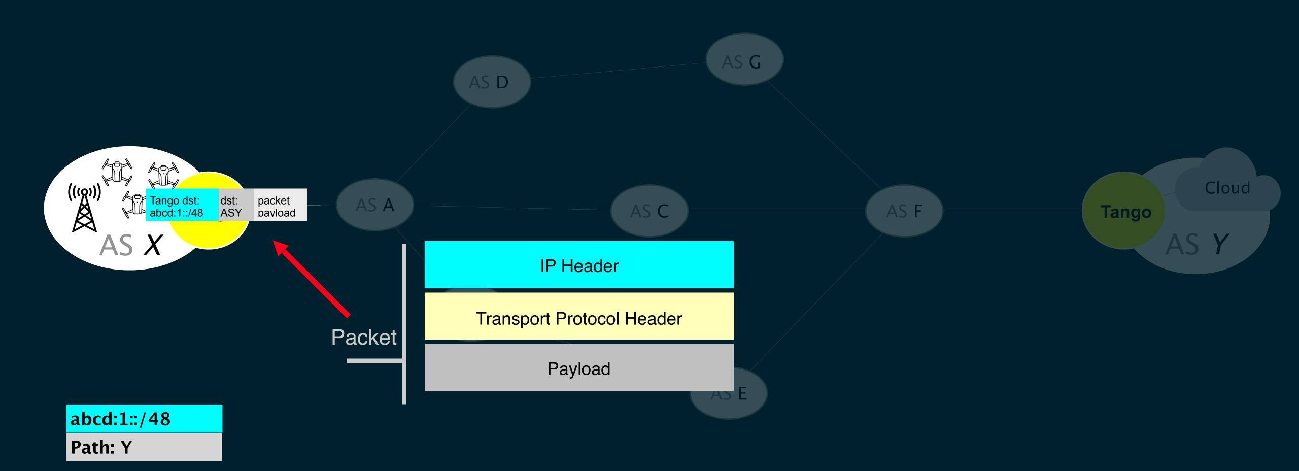
Upon reception of a packet, the sender encapsulates it with a destination within the prefix that correspond to the path of choice
